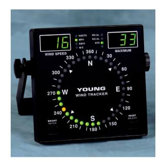
Multicolored segments give a quick visual indication of current direction and direction variability. Front panel brightness control allows adjustment for best viewing in any light.
