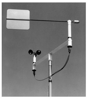
Microvanes employ a lightweight, highly responsive, expanded polystyrene (EPS) fin with a durable, UV resistant coating. For greater durability, the 12005 and 12305 Models have a thin aluminum fin. Aluminum fin models are somewhat less sensitive than the EPS fin models.
